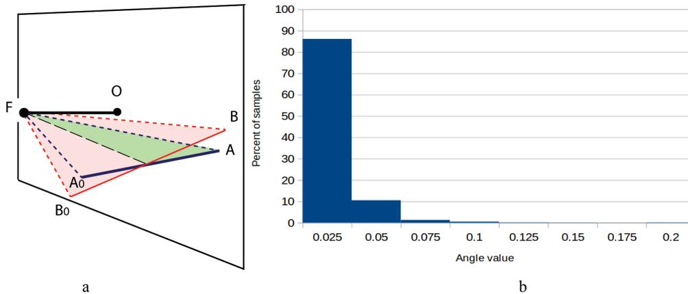
Figure 6. a. Illustration of two planes involved in error calculation.  $FO$  – the focal length of the camera ( $FO$  is normal to the frame plane),  $B_0B$  - real road position,  $A_0A$  - road position found by the algorithm.
